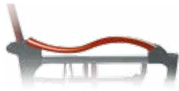
S-Ergo Seating System The unique seating system can release pressure, stabilize posture, and reduce sliding.
